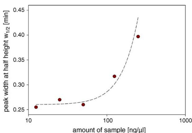
Fig. 10. Loading study on monolith **20** using albumin, 12.5–250 ng. Chromatographic conditions: mobile phase: (A) 95% water, 5% acetonitrile, 0.05% TFA, (B) 20% water, 80% acetonitrile, 0.04% TFA; gradient: 0–30 min 29–33% (B); 33–90% (B) within 5 min; flow 1  $\mu\text{l}/\text{min}$ ; 25  $^{\circ}\text{C}$ ; detection, UV 190 nm.
