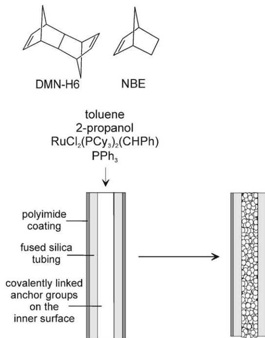
Scheme 1. Synthesis of monolithic capillary HPLC columns via ROMP.
