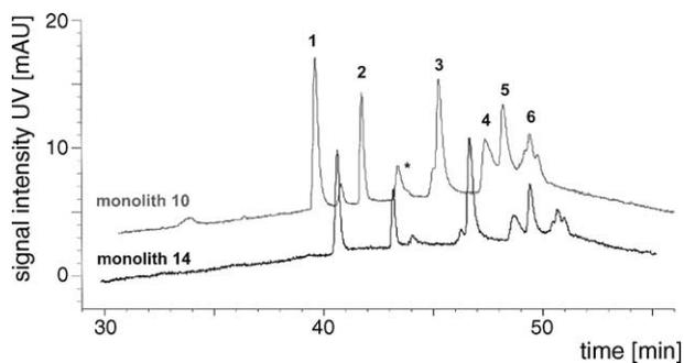
Fig. 7. Separation of the protein standard on monoliths **10** and **14**. (1) Ribonuclease A, (2) insulin, (3) lysozyme, (4) albumin, (5) myoglobin and (6)  $\beta$ -lactoglobulin, \*ghost peak, 2–8 ng of each protein. Chromatographic conditions: mobile phase: (A) 95% water, 5% acetonitrile, 0.05% TFA, (B) 20% water, 80% acetonitrile, 0.04% TFA; gradient: 0–30 min 0–60% (B); 60–90% (B) within 5 min; flow 1  $\mu$ l/min; 25  $^{\circ}$ C; detection, UV 190 nm.
