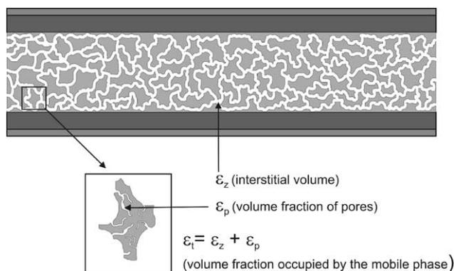
Fig. 4. Illustration of the physical meanings of the interstitial volume ( $\epsilon_z$ ), the volume fraction of pores ( $\epsilon_p$ ) and the volume fraction occupied by the mobile phase ( $\epsilon_t$ ).
