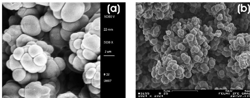
Fig. 9. Electron micrographs of (a) analytical monolith 3 mm i.d. borosilicate glass column (reprint in part with permission from [47]. Copyright (2005) American Chemical Society), scale bar corresponds to 2  $\mu\text{m}$  and (b) capillary monolith 200  $\mu\text{m}$  i.d. fused silica column, scale bar corresponds to 5  $\mu\text{m}$ .
