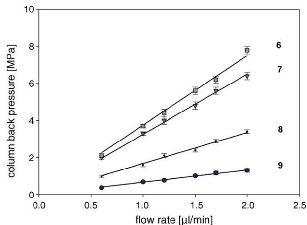
Fig. 6. Effective back pressure vs. flow rate for monoliths **6–9**. Mobile phase: water. For their synthesis, refer to Table 2.
