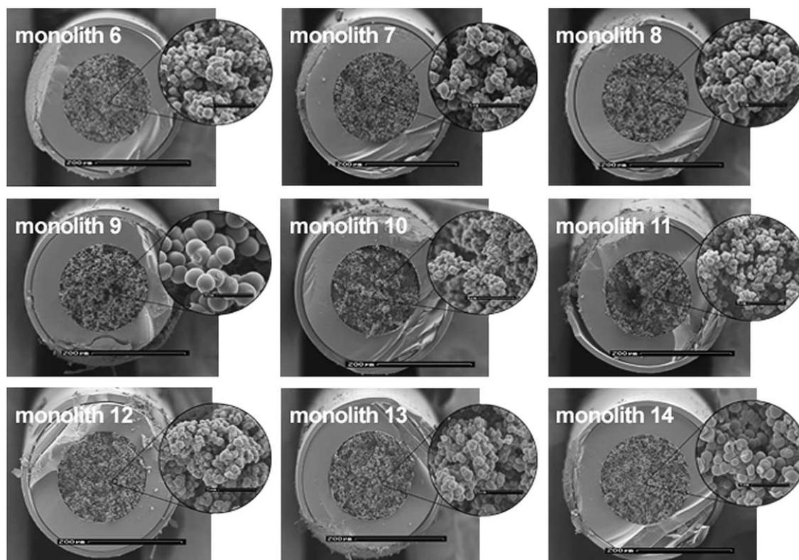
Fig. 5. Electron micrographs of monoliths **6–14**. The scale bar corresponds to 200  $\mu\text{m}$  (5  $\mu\text{m}$  in the inset). For their synthesis, refer to Table 2.
