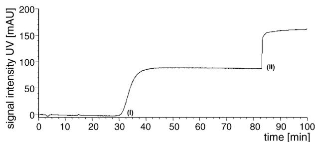
Fig. 11. Breakthrough curve for albumin recorded on monolith **18**. (I) change of 100% mobile phase A to 100% mobile phase B, (II) point of breakthrough. Chromatographic conditions: mobile phase: (A) 95% water, 5% acetonitrile, (B) 95% water, 5% acetonitrile, 0.05% TFA, 0.25 mg/ml BSA; flow 1  $\mu\text{l}/\text{min}$ ; 25  $^{\circ}\text{C}$ ; detection, UV 190 nm.
