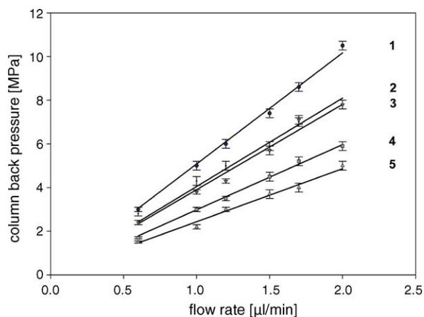
Fig. 3. Effective back pressure vs. flow rate for monoliths 1–5. Mobile phase: water. For their synthesis, refer to Table 2.
