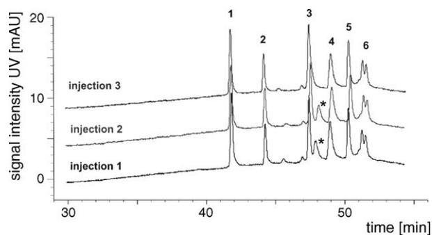
Fig. 2. Run-to-run precision of the protein standard on monolith 3, three-fold injection. (1) Ribonuclease A, (2) insulin, (3) lysozyme, (4) albumin, (5) myoglobin and (6)  $\beta$ -lactoglobulin, \*ghost peak, 2–8 ng of each protein. Chromatographic conditions: mobile phase: (A) 95% water, 5% acetonitrile, 0.05% TFA, (B) 20% water, 80% acetonitrile, 0.04% TFA; gradient: 0–30 min 0–60% (B); 60–90% (B) within 5 min; flow 1  $\mu$ l/min; 25  $^{\circ}$ C; detection, UV 190 nm.
