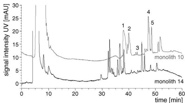
Fig. 8. Separation of the tryptic digest of cytochrome C on monoliths **10** and **14**. (1)–(5) fragments, 120 ng of cytochrome C. Chromatographic conditions: mobile phase: (A) 95% water, 5% acetonitrile, 0.05% TFA, (B) 20% water, 80% acetonitrile, 0.04% TFA; gradient: 0–30 min 0–50% (B); 50–90% (B) within 5 min; flow 1  $\mu$ l/min; 25  $^{\circ}$ C; detection, UV 190 nm.
