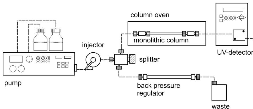
Fig. 1. Experimental setup for self-made cap-HPLC.
